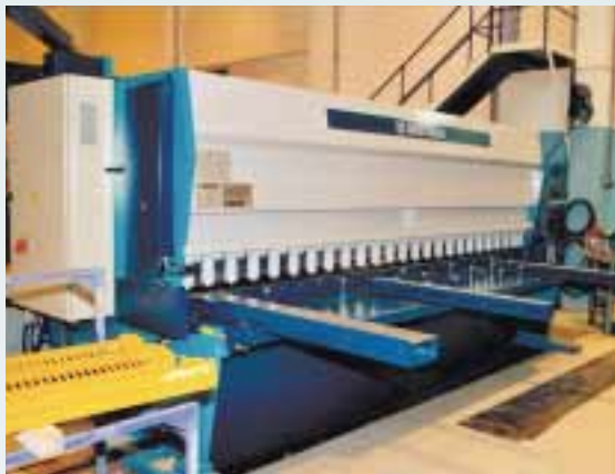
Shear model GSA 440. Cutting capacity 10 mm, cutting length 4 metres in material with tensile strength 500 N/mm 2 .
