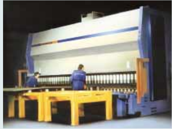
GSB model 965 delivered to Smidesbolaget in Degerfors. Cutting capacity 45 mm, cutting length 6.5 metres.
