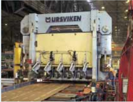
GSC delivered to SSAB in Oxelösund. Cutting capacity corresponding to about 70 mm, cutting length 3.5 metres in material with tensile strength 500 N/mm 2 .
